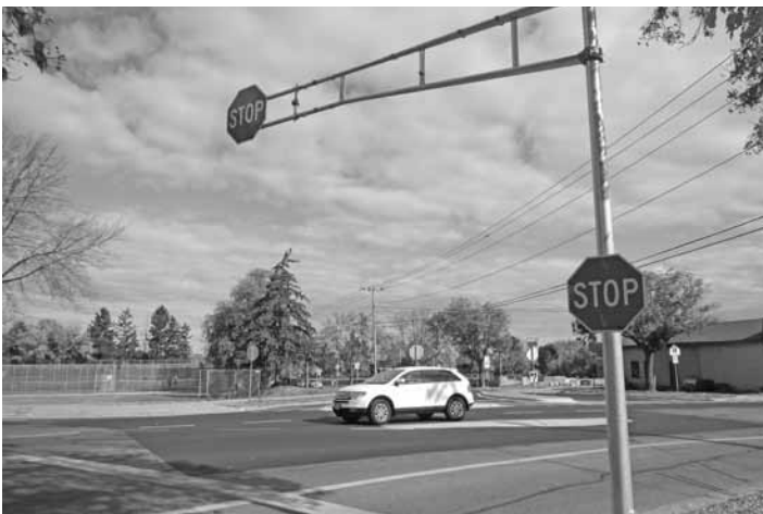
The addition of the overhead stop sign on Speedway and advance of the stop line by 20 feet slows traffic into the intersection, making it easier for drivers to turn down Highland.
